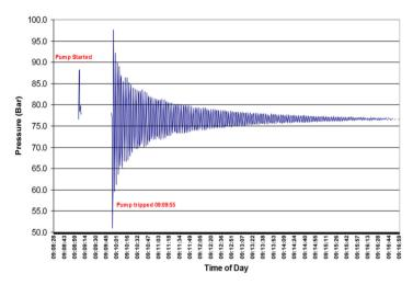
The graph shows the effects of water hammer in a Mine pump station, with an under ground pump station of 786m m static head when 2 pumps tripped.
